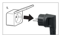
Finish charging process following the user manual of the vehicle and disconnect grid plug and vehicle connector
