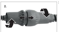
2. Unscrew the power cable separation point anticlockwise. Choose a suitable mains plug type (see below).
