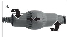
4. Tighten the power cable separation point clockwise until it audibly clicks into place and the gap between the two parts is completely closed.
